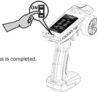
3. When the LED on the receiver becomes solid, the binding process is completed.
